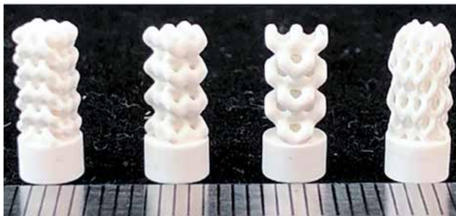
Skoltech researchers used function representation modeling and laser stereolithography to fabricate ceramic implants featuring complex internal pore structures. The first design on the left (BI001) showed highest compressive strength.
