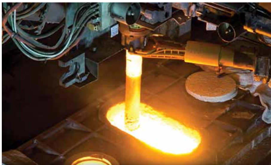
In continuous steel casting, ceramic powders help keep the liquid metal from oxidizing. Potassium carbonate may serve as an alternative and less expensive material from which to make powders.
