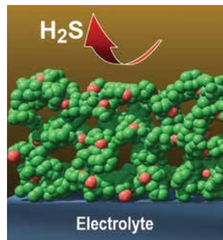
Figure 2. Schematic representation of a new class of high performing, electrically conductive, and catalytically active ceramic electrodes that tolerate carbon and sulfur.
