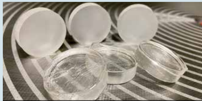
DCM Tech automated rotary surface grinders can be used to grind flat glass to precise dimensions before polishing, significantly reducing intermediate lapping steps as well as preventing breakage of what is often a high-value product. Above, glass discs before and after grinding. Credit: DCM Tech
