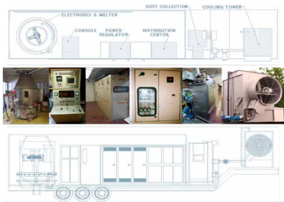
Figure 1. Design of the Melt Mizer portable testing system.
