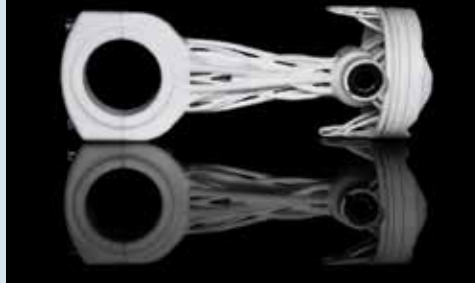
The additively manufactured piston. Credit: XJet/SPA
