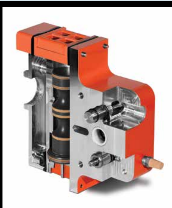
The Wilden Pro-Flo SHIFT Air Distribution System revolutionizes AODD pump operation through a design that reduces air consumption by up to 60% when compared to competitive models. Credit: Wilden
