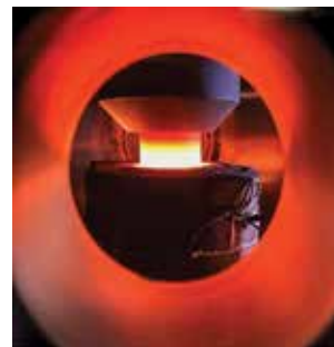
Left, schematic representation of high-entropy MXenes \text{TiVNbMoC}_3 or \text{TiVCrMoC}_3 discovered by our group in 2021. Right, MXenes being brought to ultrahigh temperatures ( > 2,000^\circ\text{C} ) in a graphite die placed in a spark-plasma sintering equipment.
