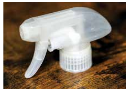
Figure 2. rGF thermoplastic pellets in injection molded commercial sprayer head.
