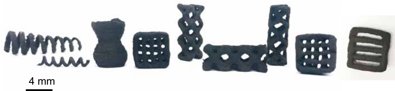
Figure 2. Several of the printed polymer-derived ceramic structures.
