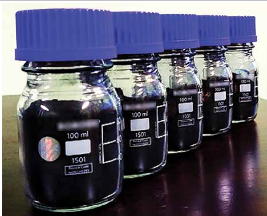
Bottles containing exfoliated graphene obtained from a new method based on plasma spraying. Reprinted with permission from Islam et al., ACS Nano , Vol. 15 Iss. 1 (1775–1784). Copyright 2021 American Chemical Society.
