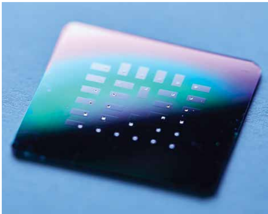
A silicon chip with 30 individual glucose micro fuel cells, seen as small silver squares inside each gray rectangle.
