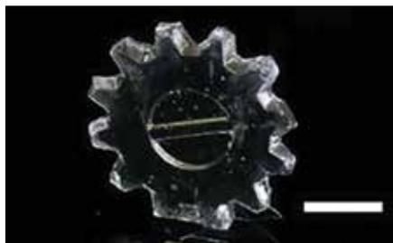
**Example of an injection molded transparent ceramic shaped like a gear. Scale bar: 5 mm.**
