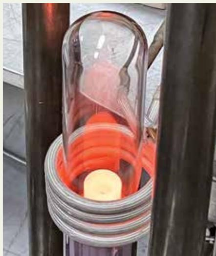
**Figure 1. Prototype induction heating testbed for melting lunar regolith simulants in a graphite crucible.**
