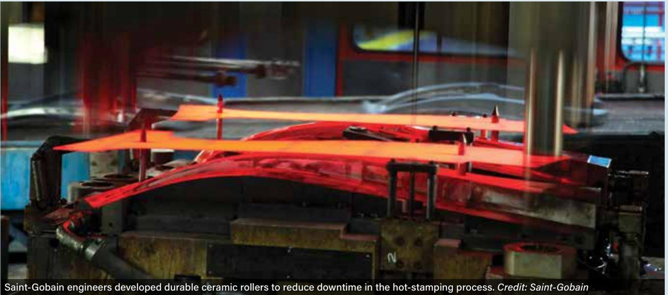
Saint-Gobain engineers developed durable ceramic rollers to reduce downtime in the hot-stamping process. *Credit: Saint-Gobain*
