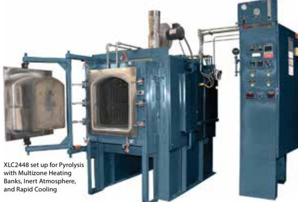
XLC2448 set up for Pyrolysis with Multizone Heating Banks, Inert Atmosphere, and Rapid Cooling
