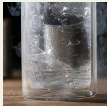
Figure 1. A collapsible hydrogen storage bladder in liquid nitrogen demonstrates its ability to repeatedly bend and fold in cryogenic conditions.
