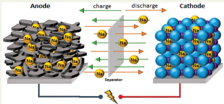
Illustration of a sodium-ion battery, one of the alternative battery compositions that may replace lithium.<sup>3</sup>
