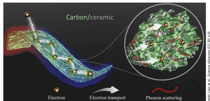
Schematic of a flexible carbon/silicon nonwoven composite created at the University of Bayreuth that exhibits low thermal and high electrical conductivities.
