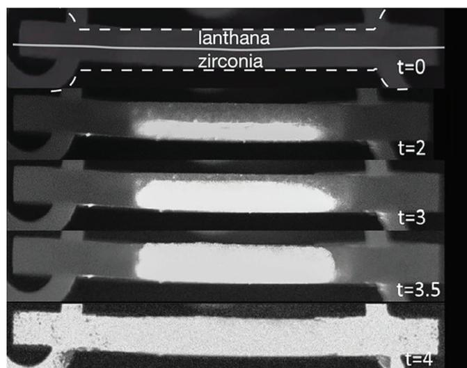
The progression of flash sintering on a lanthana–zirconia bilayer in an 800°C furnace with 300 V/cm field applied and current limited to 100 mA/mm<sup>2</sup>.
