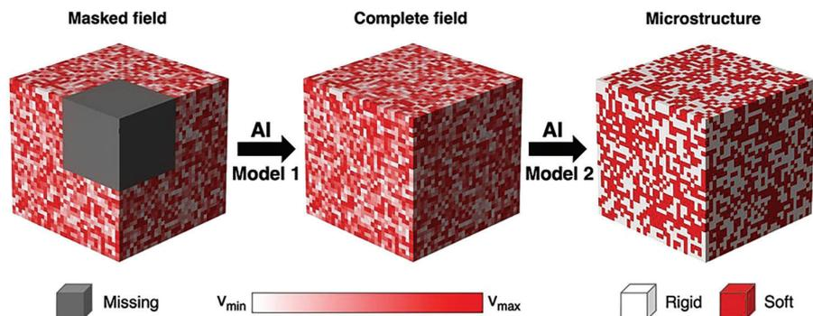
**General schematic of the deep learning method developed by the MIT researchers to predict a material’s internal microstructure based solely on its external surface characteristics. An AI model fills in the unknown parts of a partial field (gray box) while a second AI model uses the recovered complete field information to reversely obtain the corresponding microstructure.**
