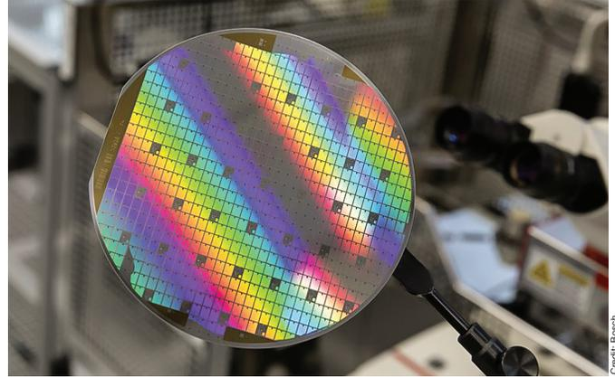
**A silicon carbide power semiconductor from German company Bosch. To prepare for an expected surge in demand for SiC electronics, several semiconductor manufacturers have announced plans to construct new or expand existing fabrication facilities.**
