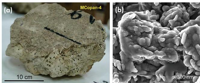
(a) A Maya plaster sample corresponding to a fine two-layer plaster floor from the mid-Classic period (500–700 CE). (b) A field emission scanning electron microscope image of the sample showing its nanogranular structure.
