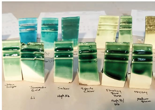
Example of various copper glazes. Researchers in the Republic of Korea recently demonstrated the potential of copper-glazed ceramic tiles to maintain long-lasting antibacterial efficiency.
