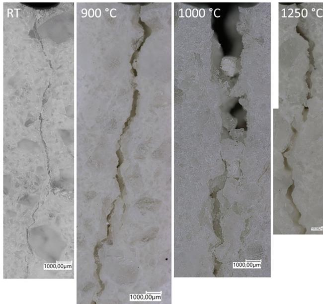
**Figure 5.** Example of research conducted at *Forschungsgemeinschaft Feuerfest e. V.* This image, which shows the crack path at different temperatures for fused silica bricks, is from a study on the fracture behavior of refractory materials up to service temperatures.
