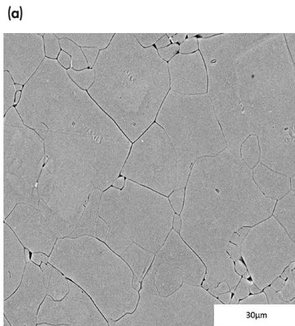
Figure 4. The SEM micrograph (a) and XRD patterns (b) of  $\text{Na}_{0.5}\text{Bi}_{0.5}\text{TiO}_3$  platelets and crystallographically textured  $(\text{Na,K})_{0.5}\text{Bi}_{0.5}\text{TiO}_3\text{-BaTiO}_3$  system studied by Entekno Materials Co.
