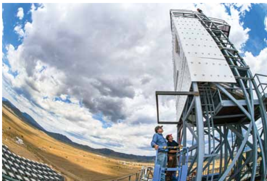
Technologists John Kelton and Daniel Ray inspect the falling-particle receiver during a cloud day atop the National Solar Thermal Test Facility at Sandia National Laboratories.
