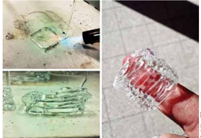
Micron3DP’s patent-pending process 3-D prints molten glass into layered architectures.
