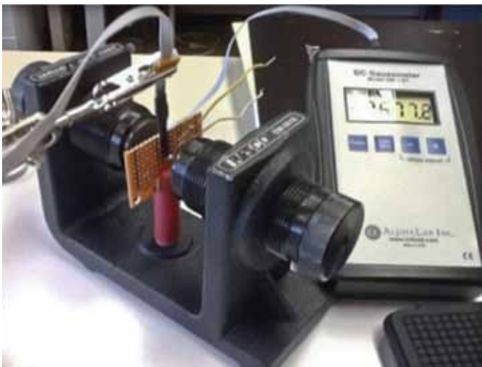
Experimental setup to determine the effects of a magnetic field on the current-voltage characteristics of a varistor.
