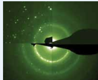
Transmission electron microscopy image showing various levels of crystallinity embedded in the amorphous matrix of the alloy.
