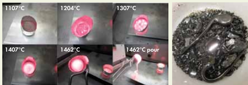
(left) Melt series based on chemistry of melted amphibolite composition from the Broborg site. Melting in atmosphere and without the use of bellows required heating the material to temperatures >1,400°C, which is not likely to be reached in ancient times. (right) Final glass produced from the melting study.
