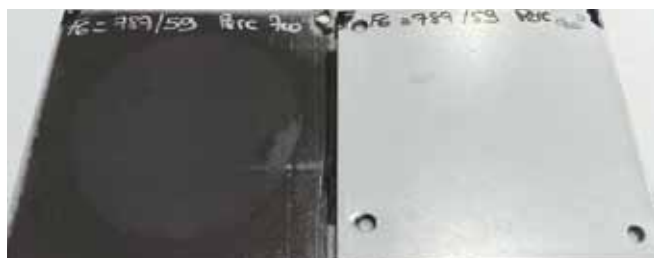
Figure 1. White enamel NPD787/F6 applied over (left) enamel primer or (right) ground coat and fired at 700°C for 4 min.
