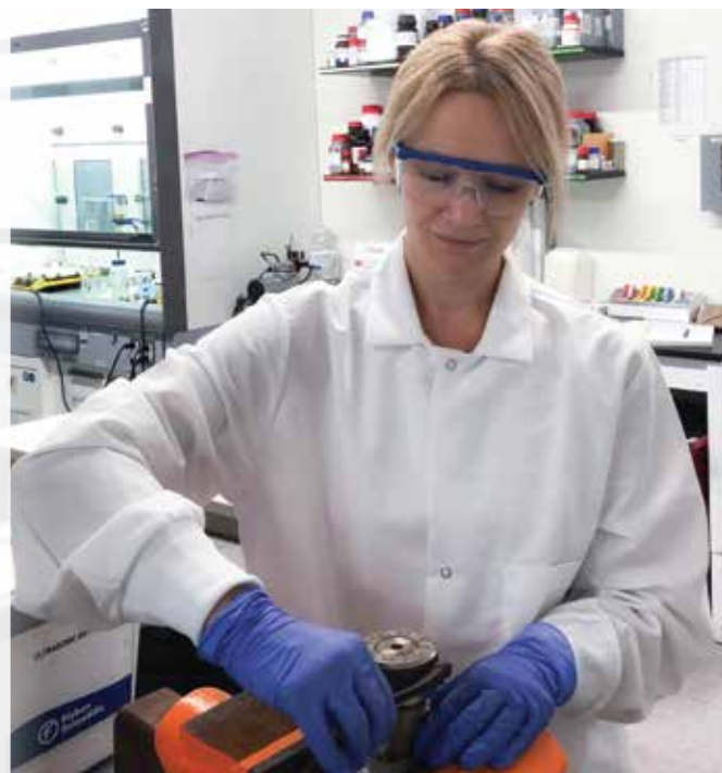
Figure 3: Pomerantseva assembling an autoclave for the hydrothermal synthesis of two-dimensional oxide heterostructured materials for use as electrodes in intercalation batteries.
