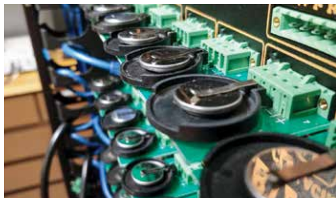
A battery cycler in Arumugam Manthiram's lab at the University of Texas at Austin for testing multiple coin cells at the same time.
