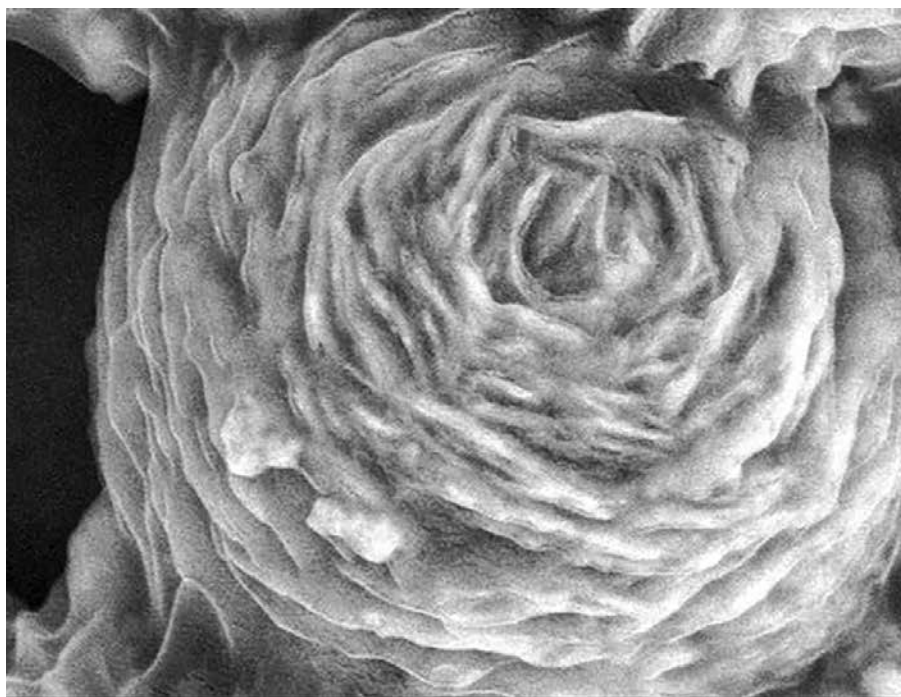
Scanning electron micrograph showing a nitrogen-doped reduced graphene oxide shell around layered bismuth-oxygen-carbon nanoplates. The microsphere traps and zaps antibiotic resistant bacteria and the resistance genes they release.
