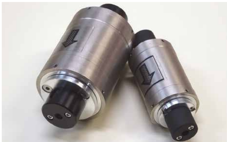
Prototype of an optical isolator using terbium yttrium oxide ceramic (right) in comparison with a commercial optical isolator based on terbium gallium garnet single crystal (left).
