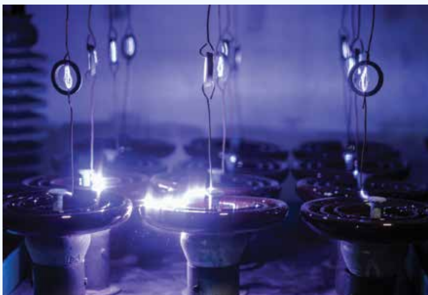
Quality control and testing at GAMMA Insulators, the utility products manufacturing subsidiary of Corona in Sabaneta, Colombia.
