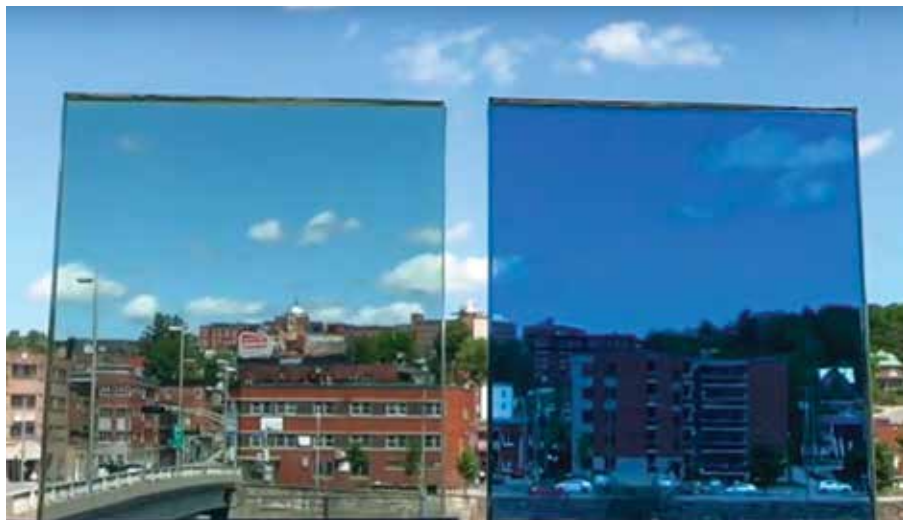
An example of thermochromic glass, a type of passive smart glass technology that changes tint in response to heat. Researchers are actively investigating the use of vanadium dioxide in such glass.
