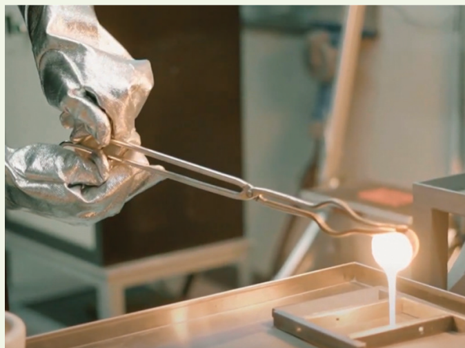
Figure 1. Modified aluminoborate glass melt for glass dissolution testing at The Pennsylvania State University.
