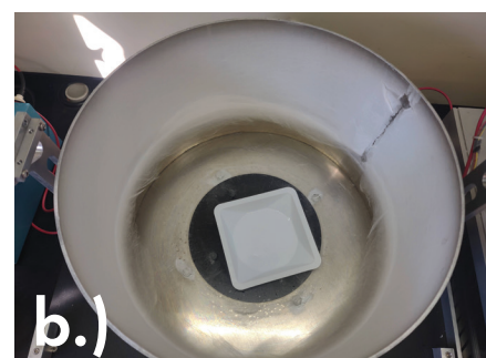
Figure 6. Improved high-throughput electrospinning setup built by The Edward Orton Jr. Ceramic Foundation. 3 (a) Main parts of the electrospinning setup. (b) A continuous fibrous mat electrospun by the system. The white tray at the bottom simply acts as a drip tray.
