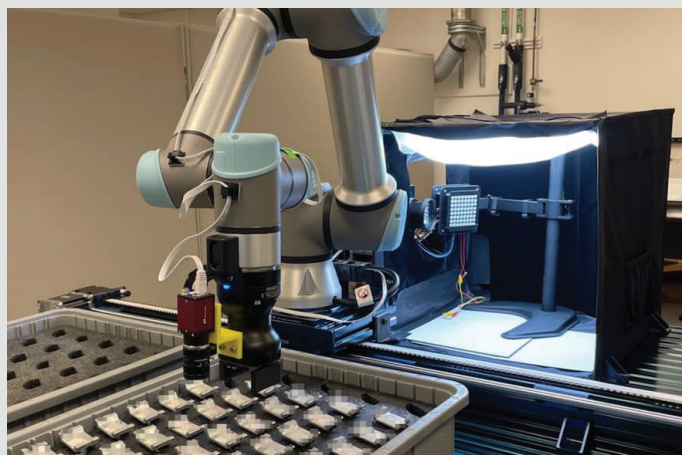
Figure 1. The GKN Aerospace project built a robotic platform that provides comprehensive parts inspection of complex metallic components.
