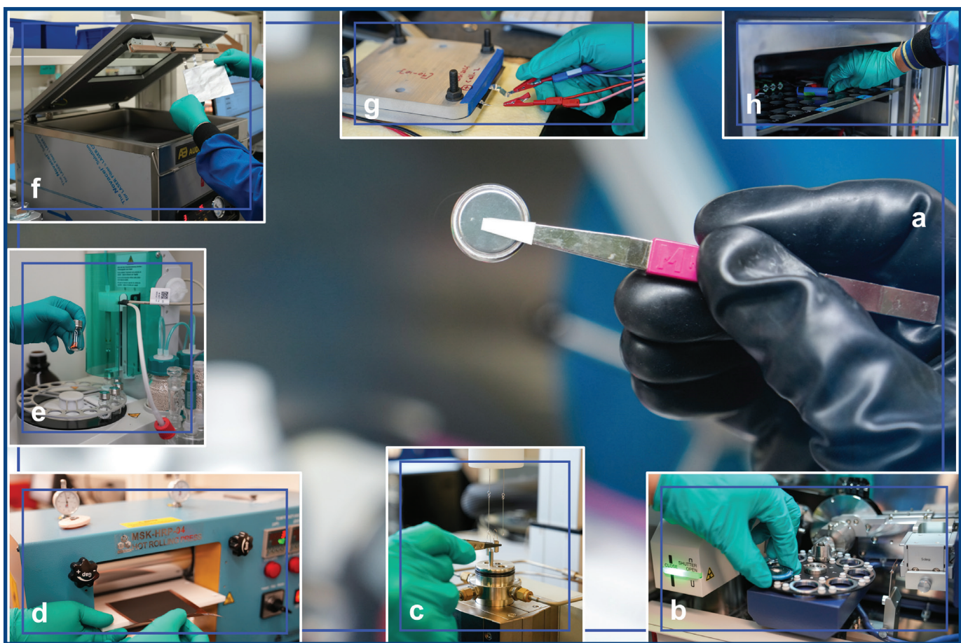
Figure 2. Some examples of the research and development capabilities at ESRI for materials performance and safety: a) in-house fabricated coin cell assembled in the dry box, b) powder X-ray diffraction sample loading, c) sample loading for thermogravimetric analysis with differential scanning calorimetry, d) calendering of in-house fabricated electrode, e) Karl Fischer moisture analysis titrator sample loading, f) vacuum sealing of in-house fabricated pouch cells, g) connecting pouch cells in pressure stacks for electrochemical testing, and h) placing an 18650 cylindrical cell in a temperature chamber for electrochemical characterization.
