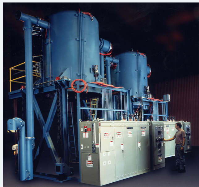
Figure 6. Series 4300 vacuum furnace for chemical vapor infiltration and graphitization. The furnace may be built in a top-loading or bottom-loading configuration.
