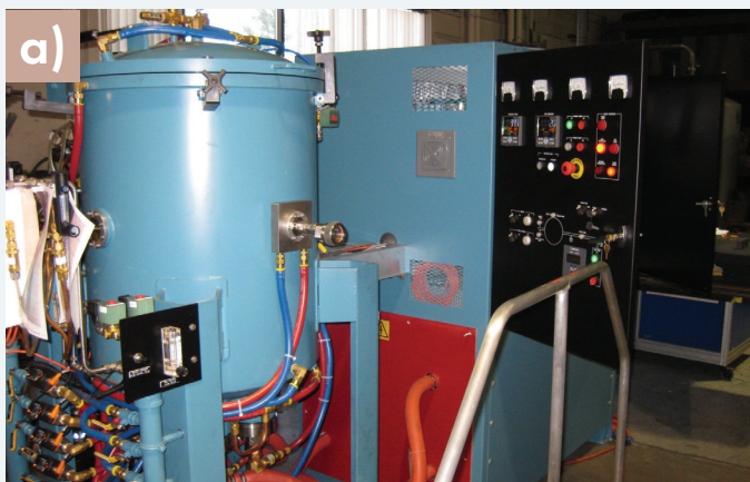
Figure 3. a) Series 45 3,200°C graphite top-loading furnace and b) top view of hot zone.
