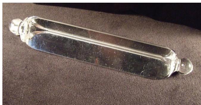
Figure 1. Soda lime silicate prism from the same time period as Newton’s optical research work. Sample currently held at the British Museum.
