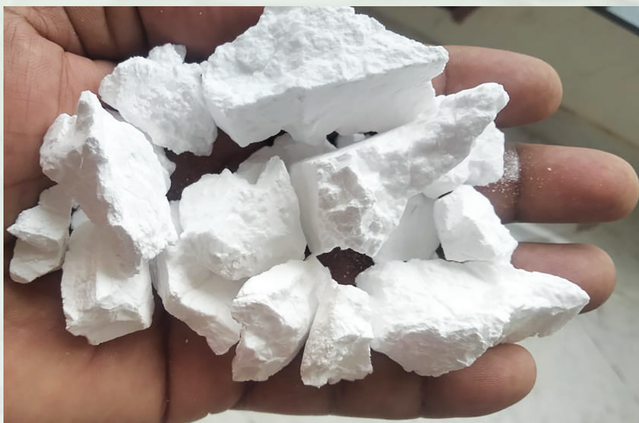
Example of the sintered cristobalite synthesized through the new rotary kiln-based method. The use of a rotary kiln means no flux is required to achieve complete transformation of the quartz into cristobalite.
