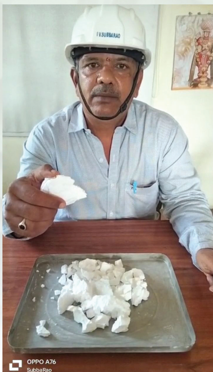
Example of the sintered cristobalite synthesized through the new rotary kiln-based method. The use of a rotary kiln means no flux is required to achieve complete transformation of the quartz into cristobalite.
