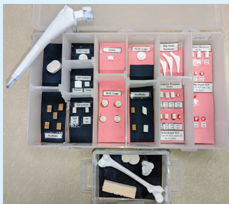
Figure 1. A collection of 3D-printed calcium phosphate parts made by Westinghouse Distinguished Chair Professor Susmita Bose and her team.
