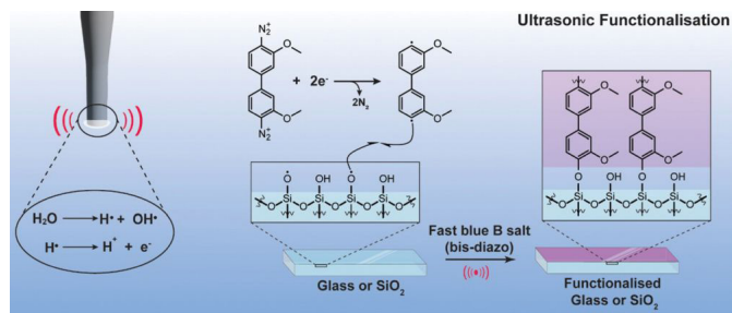
Schematic of the ultrasonic fabrication of diazonium films on glass.
