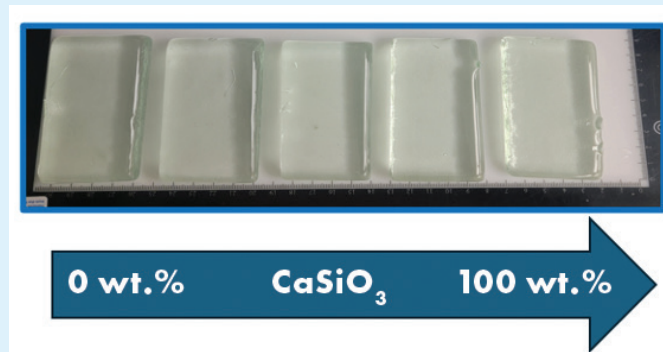
Figure 1. Container-type soda–lime–silica glasses produced with incremental substitution of the calcium-bearing raw material CaCO 3 with CaSiO 3 , from 0 wt.% (left) to 100 wt.% (right).
