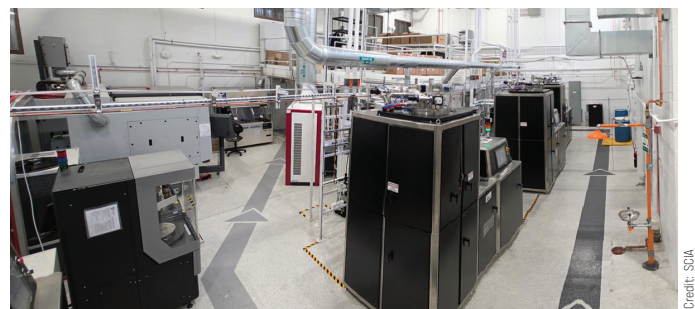
Figure 2. The onsemi Silicon Carbide Crystal Center (SiC3). It is equipped with three 150 mm and one 200 mm physical vapor transport growth furnaces, a Boule Pro 200AX CNC grinder, an ENGIS surface grinder, an Accretech edge grinder, a SOMOS IWT diamond wire cutter, a SOMOS double-side polisher, and an AXUS scrubber—enabling full industry-grade wafer production.
