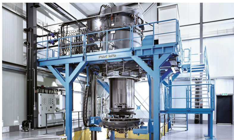
Figure 4. Example of an IVS bottom loader graphite purification solution. The flexibility of the furnace platform allows IVS to support both established and next-generation markets, and the modular design enables systems to be scaled and configured to match specific production volumes and feedstock characteristics.
