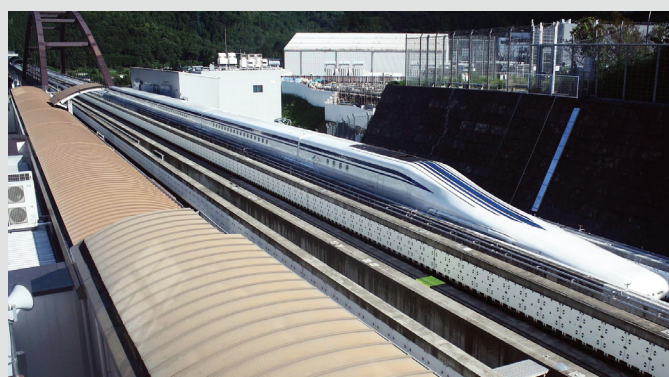
Figure 1. Photo of the Central Japan Railway Company's SCMaglev Series L0 train, which uses an electrodynamic suspension system.
